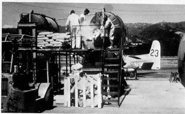
Preparing a fire-retardant mixture to be dropped on a forest fire from an air tanker, Ukiah Air Tanker Base, Mendocino County, Calif.
