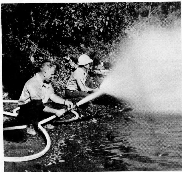
Field test of a new nozzle made from polycarbonate (Lexan). Nozzles of this material are harder than brass and one-third its cost, yet they weigh only a few pounds.
