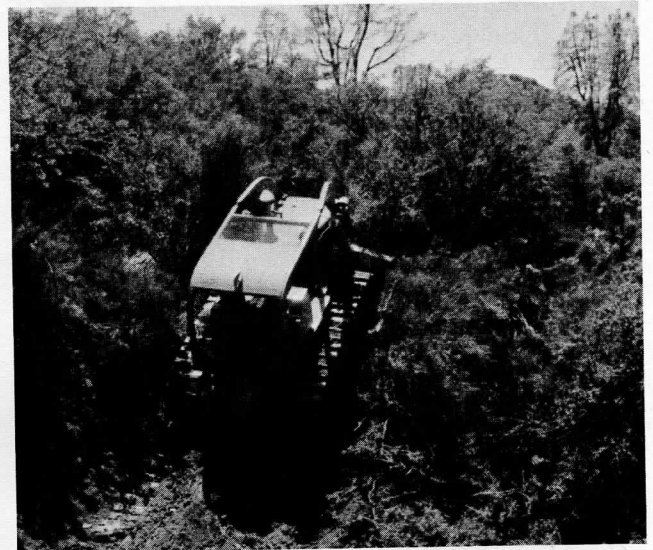
Performance tests of several makes of large and medium bulldozers were conducted during the summer. Tests included line building capability in different kinds of vegetation and topography, winching ability, and cross-country performance.
