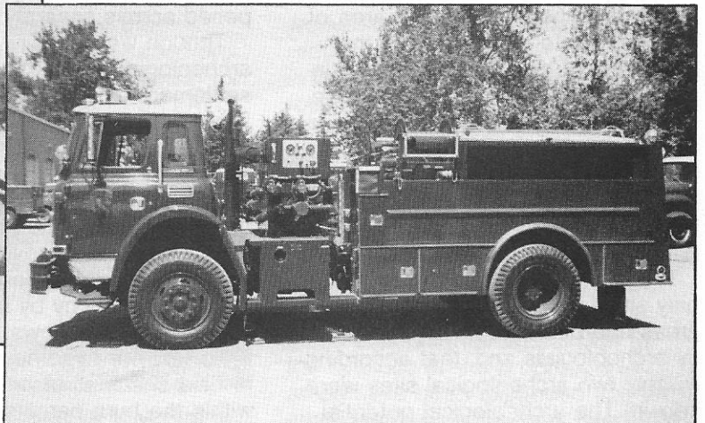
What a difference! This is pilot model #11. It is a three man conventional drive engine that holds 1100 gallons of water and has a 500 gallons per minute auxiliary pump.
