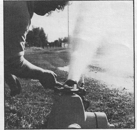
Volunteer Leslee Holmes tests the flow of a hydrant during the hydrant testing project for the Bella Vista Water District.
